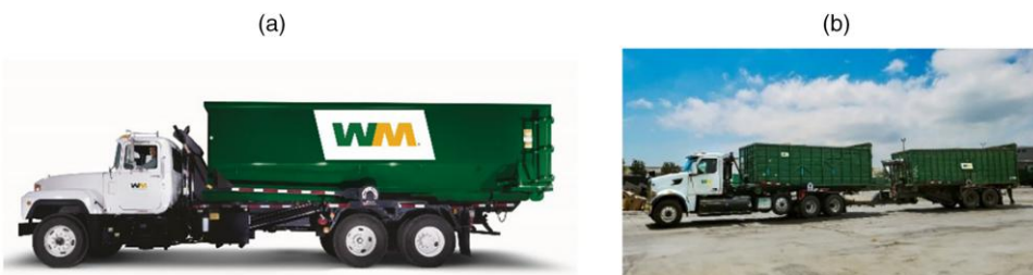
Figure 3. (a) A Regular Vehicle for Industrial Waste Collection and (b) a Tandem Vehicle with Two Containers
